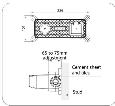
Step 1.Connect curved leg with the inlet pipe inside the wall
