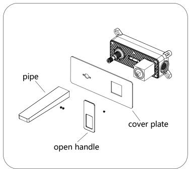
Step 3.Install shower faucet properly,and connect to curved leg on the wall
